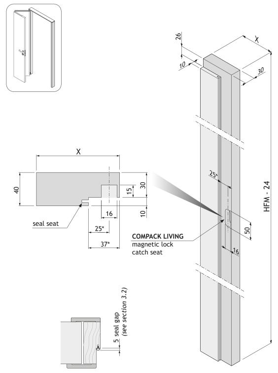
The dimension marked with (\*) vary according to the seal gap dimensions.
