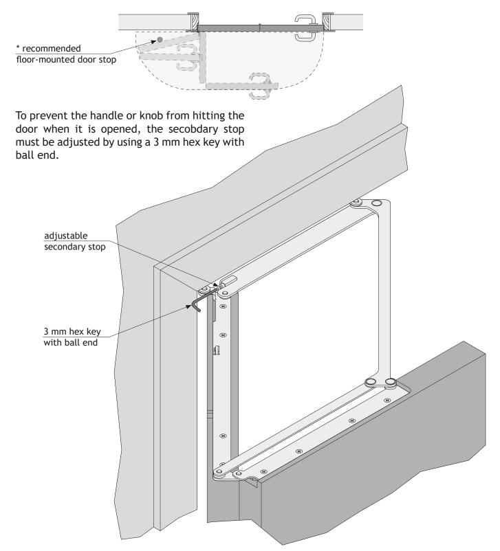
\* Important: after adjusting the stop, a floor-mounted doorstop should also be installed.
