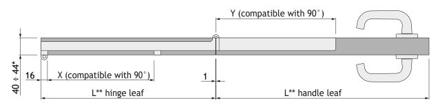
(\*\*) Hinge leaf and handle leaf widths are calculated with a reciprocal distance of 1 mm.
